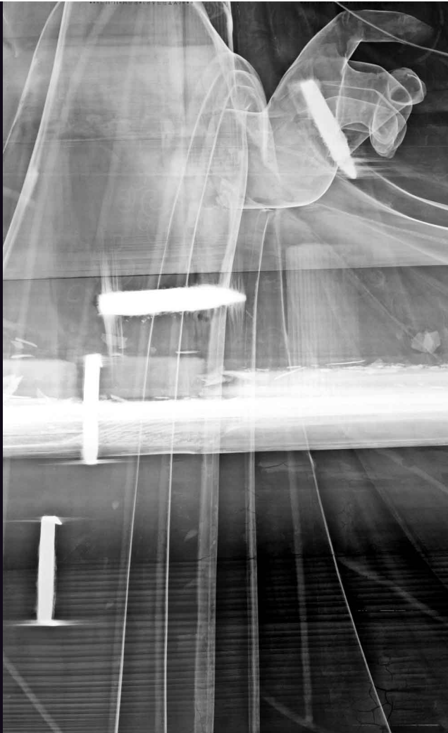
Radioscopic image of the inner structure. Pins, nails and the wooden construction are clearly visible.
