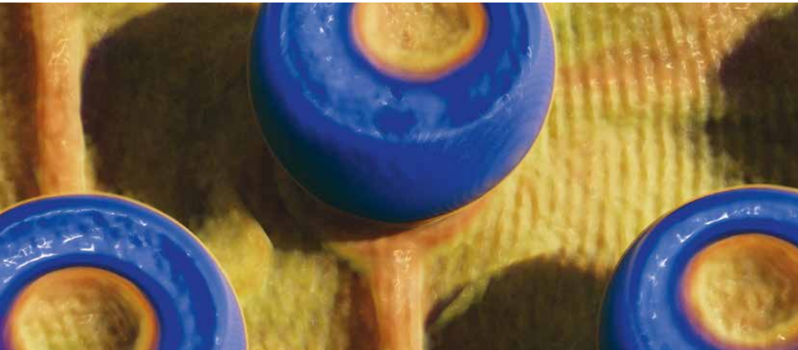
Track to pad from a BGA ball with a big void
