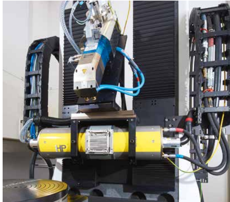
High-energy minifocus X-ray tube and high-resolution microfocus X-ray tube
