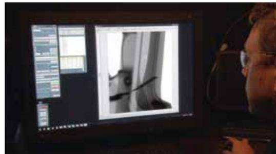
An operator reviews ADR results, choosing the part data and looking at images taken to see the individual defects provided with physical measurement, determining if they meet pass/fail criteria.
