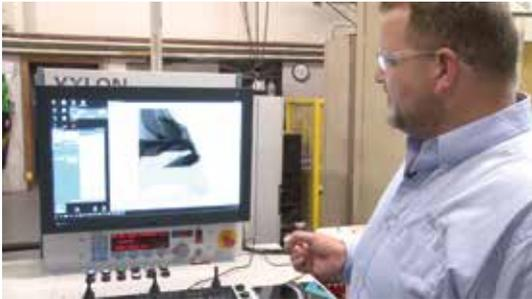
The operator can live view the part as it moves through a series of programmed views without any operator interaction once programmed.
