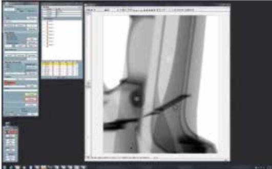
The benefits of ADR affect both the efficiency and profitability of the business. ADR provides more accurate, reliable and repeatable evaluations, and it increases the speed of inspection. It helps to reduce the operator's workload, scrap or wasted parts, and enhances the security of parts produced. In addition, the data is automatically added to the database. ADR software classifies flaws by categories and types to track the statistics to identify any trending issues. Example issues include:
