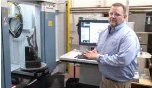
During the creation of an [instructional video now available](#), the YXLON MU60 AE is shown to inspect a large and intricate automotive cast part placed inside the system by automatic loading. (Note the doorway has dual control operation and an automatic light curtain for operational safety.)
